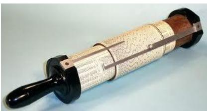
cylindrical slide rule has the scale spiralling around and around giving a much greater effective length and therefore greater accuracy.
